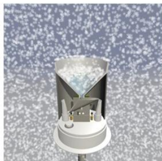
Snowflakes melt, trickle into tipping bucket
