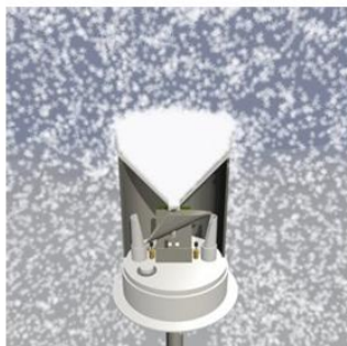
Intense snowfall overflows gauge funnel
