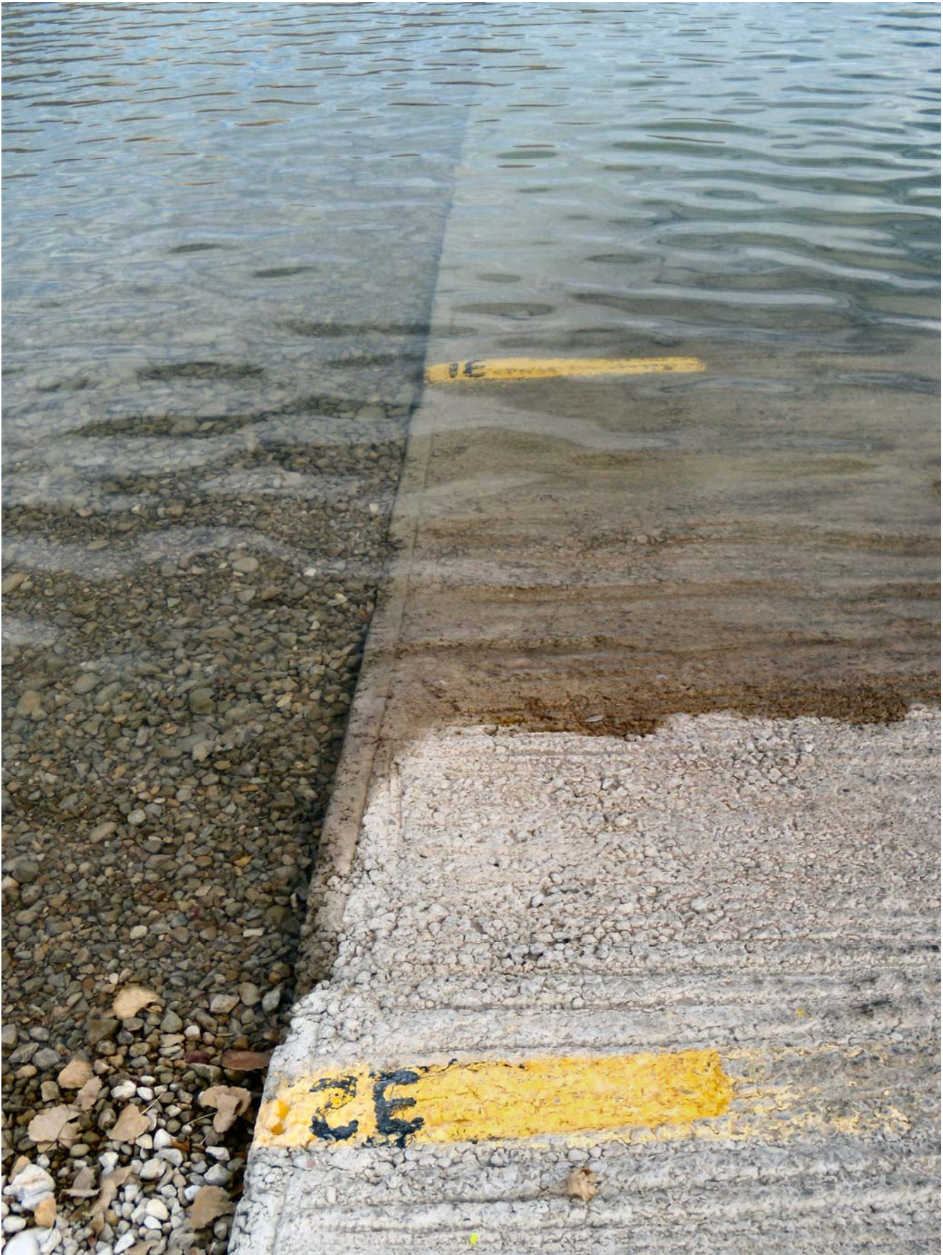
Photo 10: Painted inclined staff gage along edge of Millsite Reservoir boat ramp. EWCD website reported 31.58 feet.
