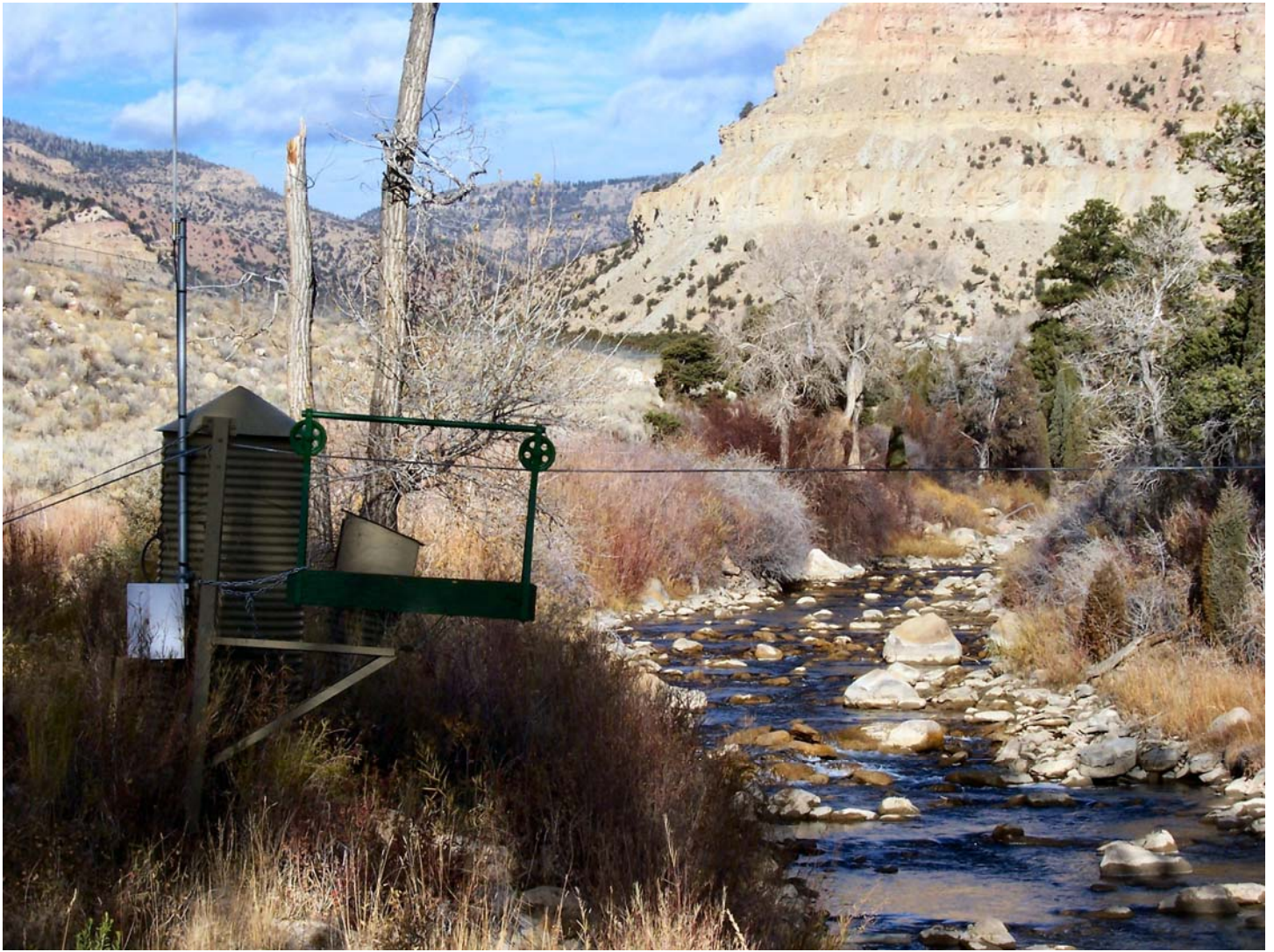
Photo 5: Huntington Creek gage, looking upstream, showing cable car.
