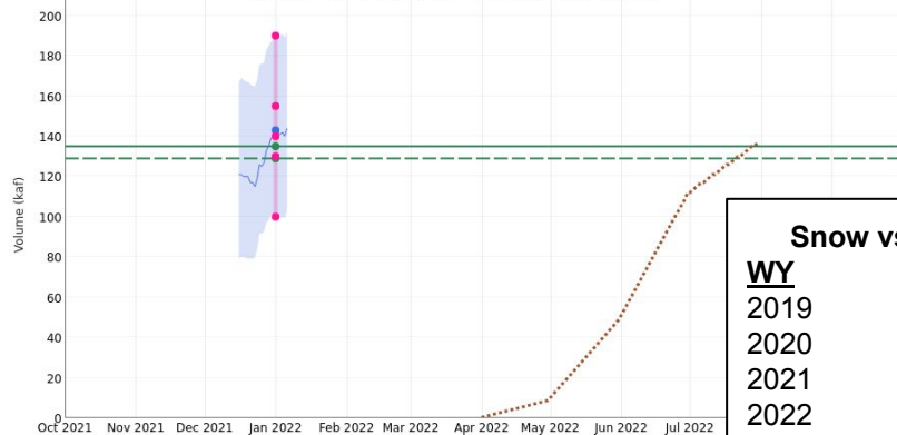
Frying Pan - Ruedi Reservoir, Basalt, Nr (RURC2) Period: Apr-Jul, Official 50% Forecast (2022-01-01): 140 kaf (104% Average, 109% Median) ESP is Unregulated and No Precipitation Forecast Included
