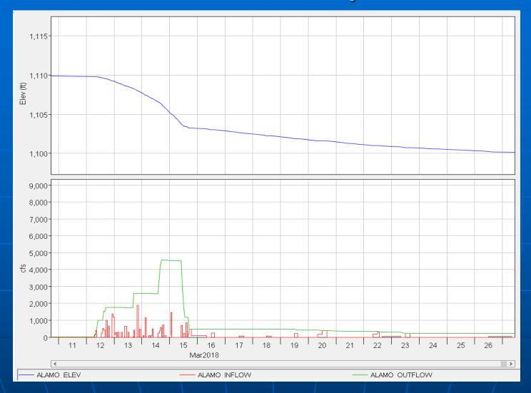
Recent drawdown to target elevation 1100 ft NGVD to facilitate a diveinspection of the outlet works intake sill. Maximum Q = 4,800 cfs
